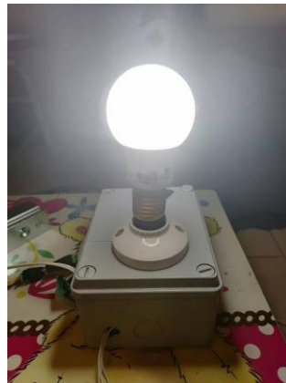
Figure 6: The lamp automatically switches ON when face was recognized by application
