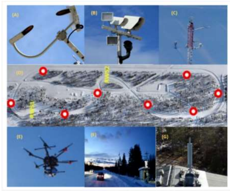
Figure 3: (A) Visibility and weather detector; (B) surface state sensor; (C) road weather station and camera; (D) test track; (E) test track equipped with IoT sensors (red spots); (F) drone; (G) field measurements in a real environment; (G) 5GTN road weather stations
