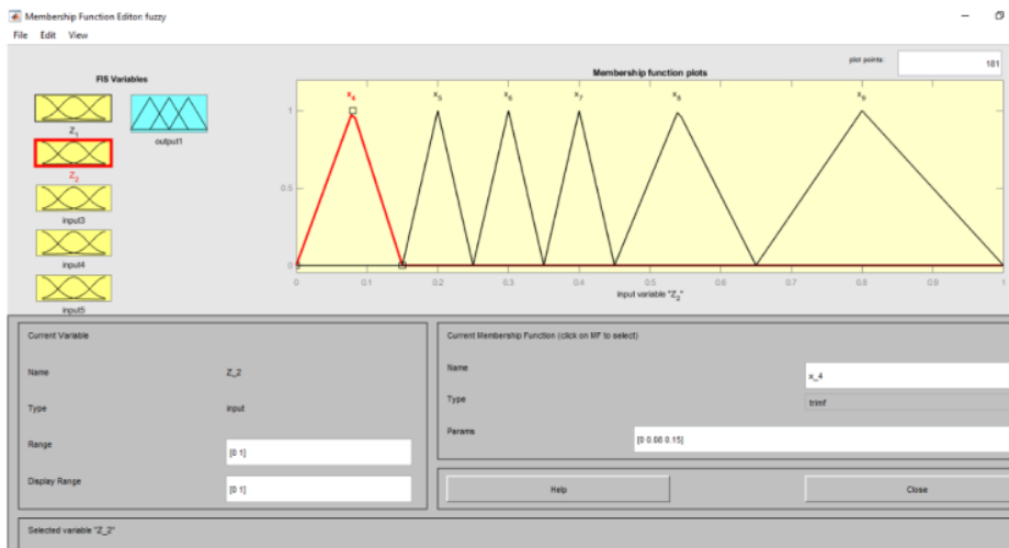
Figure 4: Representation of the input and intermediate factor of the intermediate module z_2 : functional components of the transport and logistics system of the model developed by us in the triangular form of the representation implemented in the Matlab software environment
