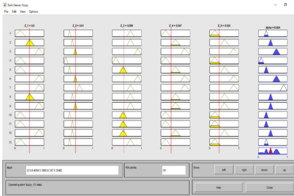
Figure 6: Defuzzification of data using the Mamdani method implemented in Matlab software is implemented
