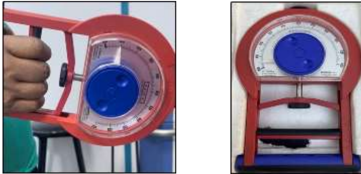
Figure (1): Maximum Grip Strength Test with Dynamometer
