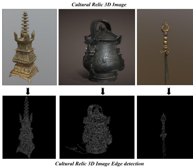
Fig. 3. Before and After Cultural Relic 3D Image Edge detection of Haihun Marquis mausoleum, Ashoka Tower, and Tibetan sacred props
