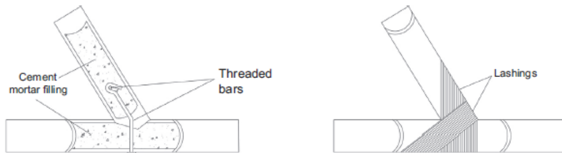
Figure 12. Connection with reinforcing steel and cement filler
