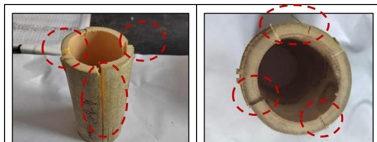
Figure 8. Progress of bamboo shear test (Taken by the author)
