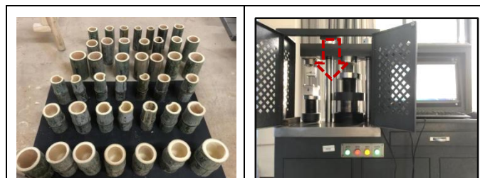
Figure 2 . The compression test process of bamboo (Taken by the author)site of
