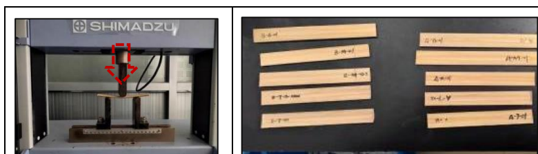
Figure 3 . The flexural strength test process and specimens(Taken by the author)
