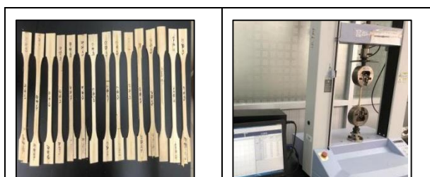
Figure 4. Processing of tensile specimens (Taken by the author)
