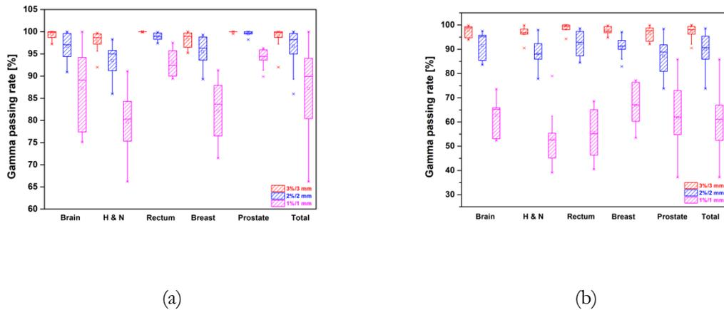
**Figure 2.** Box plots of GPRs using gamma criteria of 3%/3 mm, 2%/2 mm, and 1%/1 mm for the MapCHECK (A) and Octavius (B) devices.
