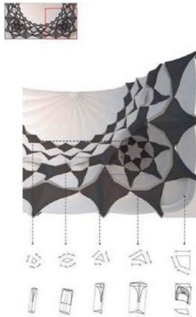
Figure 27. Damascus: Madrasa-al-Zâhirîyah, 1277. Elevation view with a geometrical analysis of the bottom layer-1 (Source: Author)
