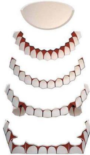
Figure 21. Damascus: Eastern entrance of the Citadel, 1214. Muqarnas dome deconstructed into its four layers (Source: Author).
